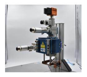
As relevant fact, NIT manufactures the fastest uncooled MWIR cameras of the market able to provide 10 kHz @ 32x32 resolution and 2 kHz @ 128x128 resolutions. NIT imagers are suitable for monitoring in real time/in line dynamics processes to a cost compatible with most industrial requirements. Regarding the second branch, at present time NIT manufactures and commercializes three solutions:
