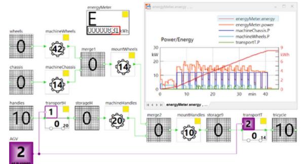
b Power and energy consumption of a (small) assembly line, Image Copyright ESI Group
